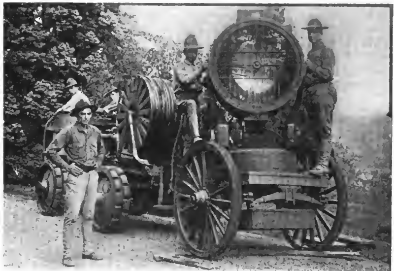
Field generator and tractor with searchlight used by the U. S. Marine Corps
